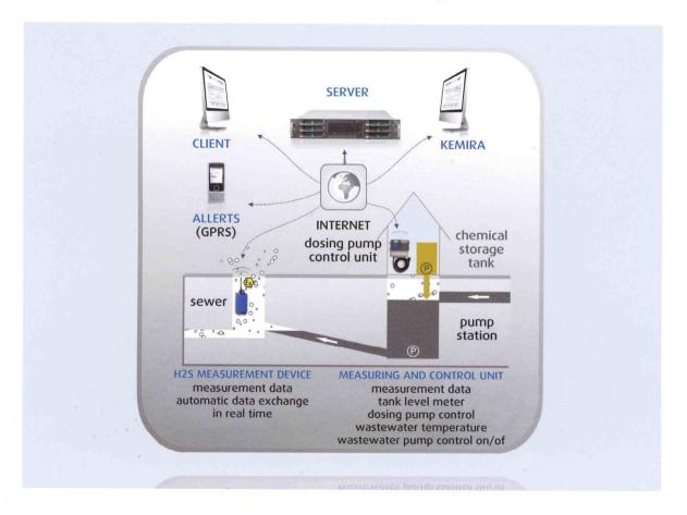
Kemira H<sub>2</sub>S-Guard is a complete system package that allows you to efficiently fight the harmful effects of hydrogen sulfide buildup.
